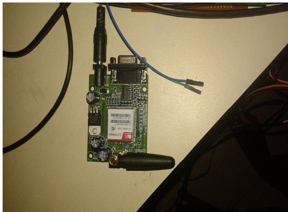
**Figure 6.4: GSM Modem**
