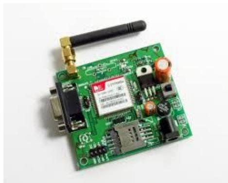
**Figure 3.6.1: GSM Modem**
